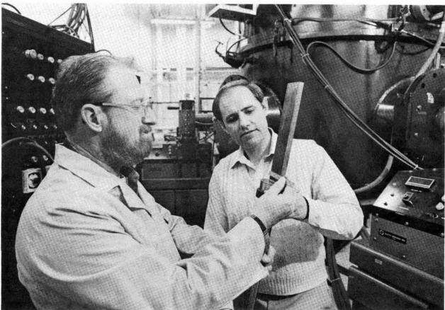
MEASURING the substrate holder are Joe Fedzuga (left) and Mark Smith (both 1834). In the right background is the low-pressure plasma spray system (LPSS) that began operations in April.
